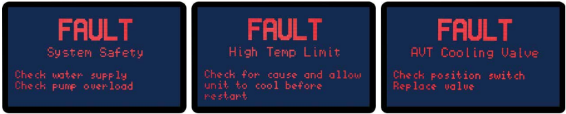
Sample of Fault display screens. Not all Fault screens are shown here. Check manual for more information.
