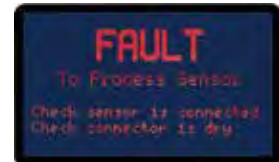
Sensor Probe Fault Screen.
