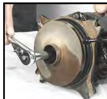
Removing impeller locking screw with ratchet
