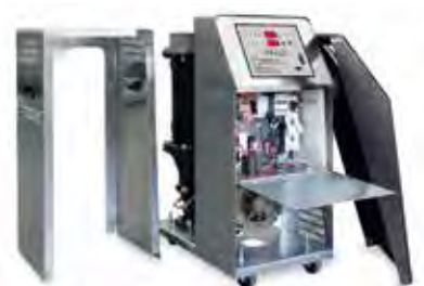
Thermoformed panel removed and electrical cabinet open.
