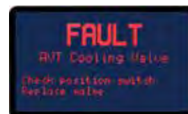
AVT Valve Fault Screen.
