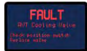
AVT Valve Fault Screen.
