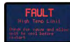
High Temp Limit Fault Screen.
