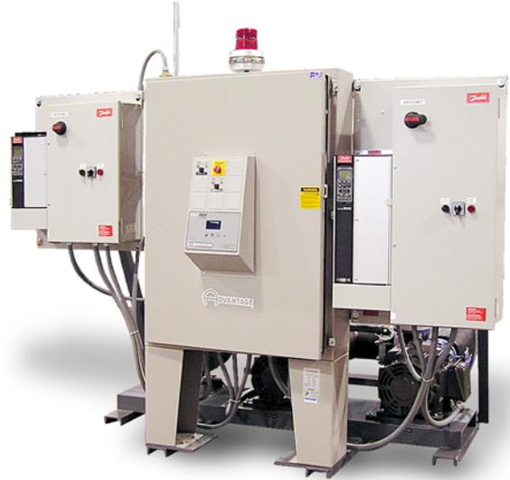
Pump station with variable speed drives. Shown with optional drive bypass to allow pumps to operate at full speed in the event of a drive failure.
