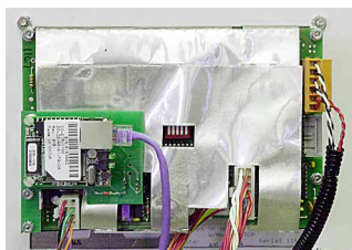
Advantage instrument with Modbus™ TCP/IP add-on circuit board.
