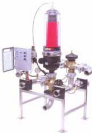
Model #ATD(1)X2-130mCW-A System is rated @ 100 GPM max. Single-pod requires city water for back-flush (40 GPM @ 50 PSI min) Pump and skid not shown.
