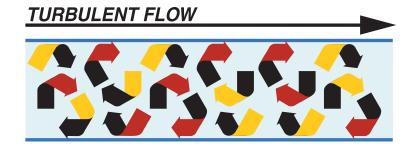
**TURBULENT FLOW** is characterized by turbulence, where fluid does not flow in smooth layers but is agitated.
