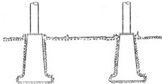
TOWER STAND MOUNTING - PIER MOUNTING
