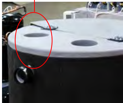
Typical reservoir lid and From Process opening.
