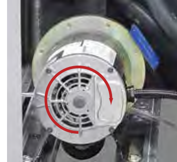
Correct shaft rotation is clockwise.
