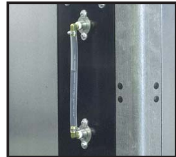
Typical reservoir sight glass Figure 3.2A
