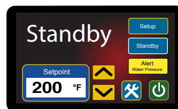
Yellow Alert Icon showing Water Pressure Fault
