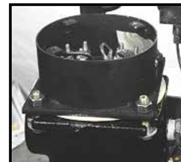
Heater mounting bolt
