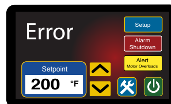
Error Screen showing Yellow Motor Overload Alert Icon
