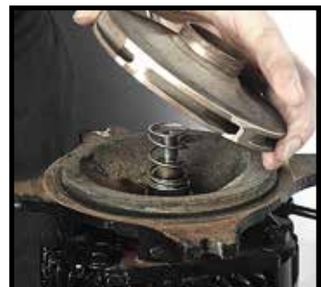
Aligning impeller and spring
