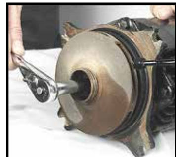
Removing impeller locking screw with ratchet
