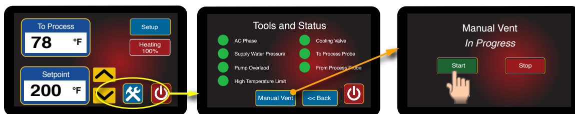
Showing the screen advance to Manual Vent.
