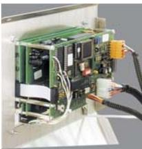
**ELECTRONIC CONTROLS MANUFACTURING...** an affiliated company, established in 1984, **ADVANTAGE Electronics, Inc.** offers complete engineering services for control instrumentation, including microprocessor programming, printed circuit board design, layout, assembly and testing. Custom programming and computer interfacing is available for special customer applications.
